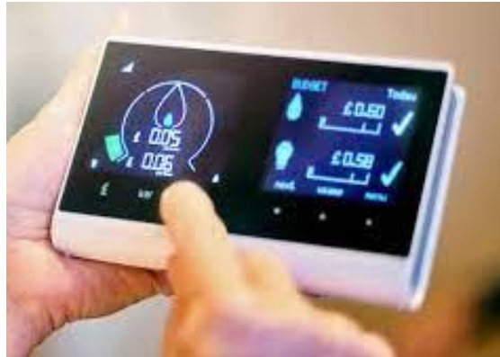
A typical In-home Display provided with smart meters
